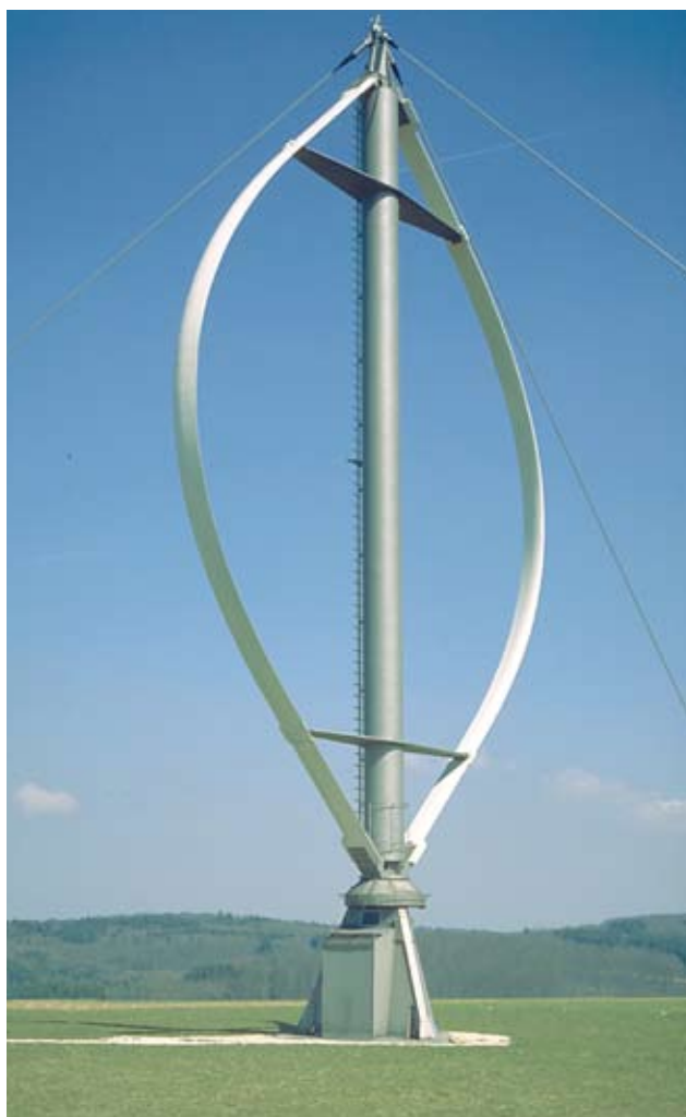
Figure 1.9 - Turbine Darrieus type
