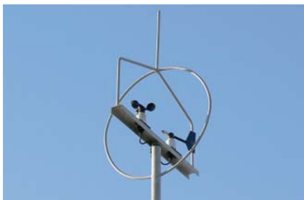
Installation of the anemometer on an anemometric tower
