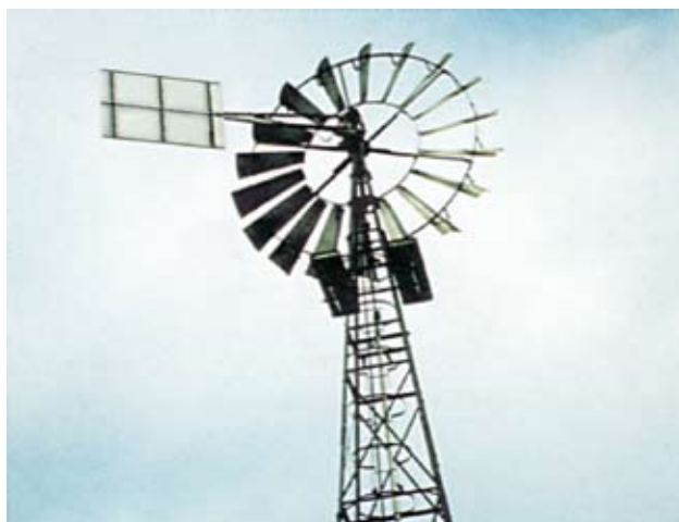
Figure 1.15 - Multi-blade turbine
