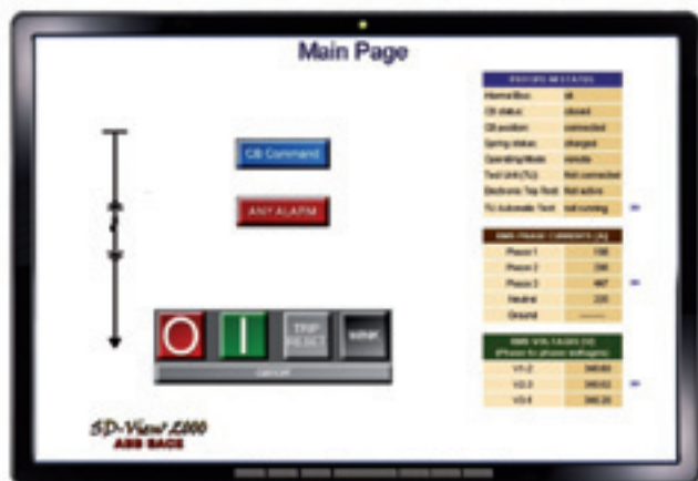
Figure 33: Main graphic page of an Emax air circuit-breaker
