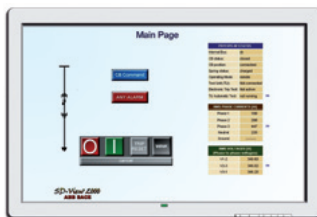
Figure 15: Example of user interface for the supervision of an electrical installation
