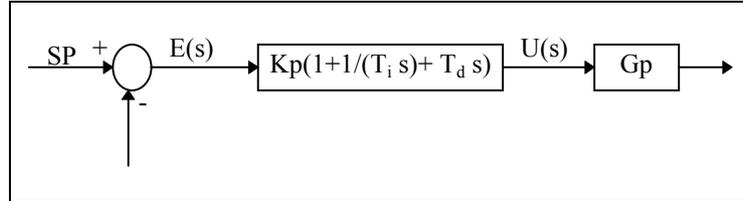
$$u(t) = K_p (e(t) + \frac{1}{T_i} \int_0^t e(\tau) d\tau + T_d \frac{de(t)}{dt}) \xrightarrow{L} U(s) = K_p (1 + \frac{1}{T_i S} + T_d s) E(s) \quad (1-4)$$
