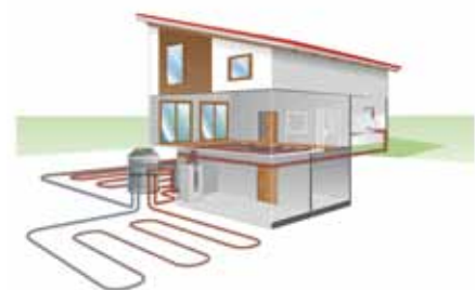
B – Heat extraction with geothermal collectors
