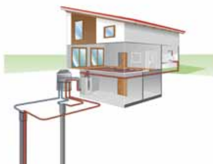
A – Heat extraction with geothermal probes
