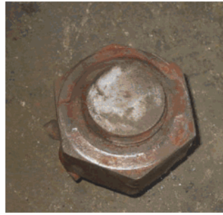
Figure 3. Appearance of pump shaft fatigue fracture surface.
