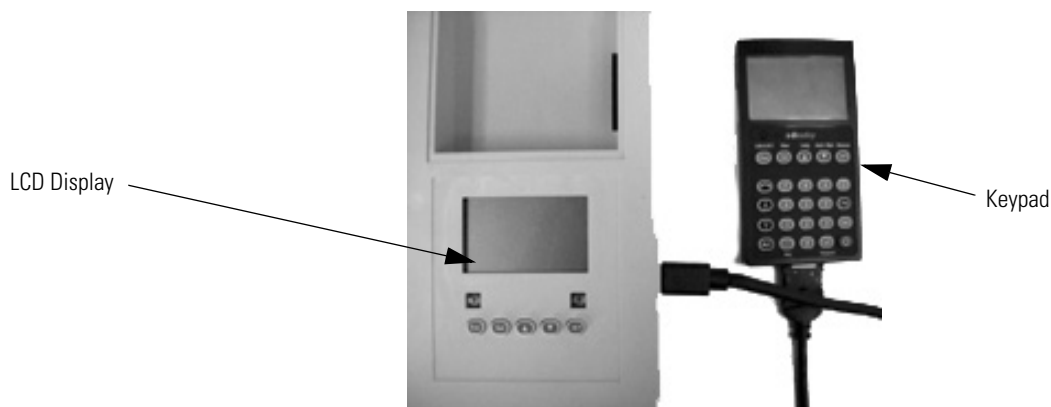
Figure 1.35: LCD Display with Keypad
