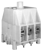
Larger amperage switches such as the non-metallic 100 amp RSWP use sintered bronze plates as the explosionproof joint.
