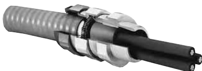
TMCX Terminator cable fittings are suitable for use with Type MC jacketed metal-clad cables with interlocked or corrugated armor and Type TC tray cable in Class I, Division 2, Groups A, B, C, and D locations. TMCX fittings are suitable for use with Type MC-HL and Type ITC-HL cable listed for use in Class I, Division 1.
