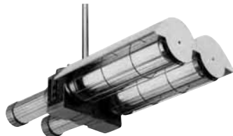
Illuminator™ EVFT fluorescent luminaires are compact and provide excellent light output for service pits. Optional polycarbonate tube protects lamp tube assemblies from overspray and impact. UL listed for Class I, Group D; also available for Class I, Groups B, C ("GB" suffix).
