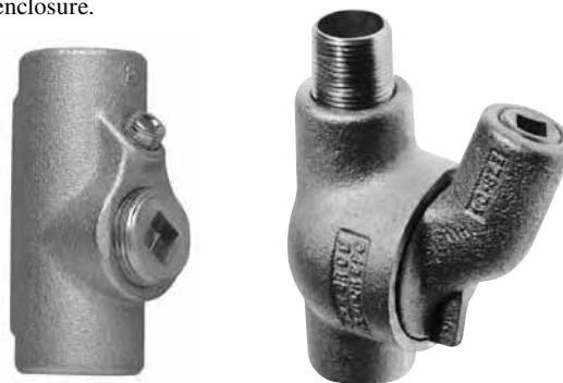
EYSX Series – For sealing in vertical or horizontal conduit runs. Class I, Groups A, B, C, D, and Class II, Groups E, F, and G.
