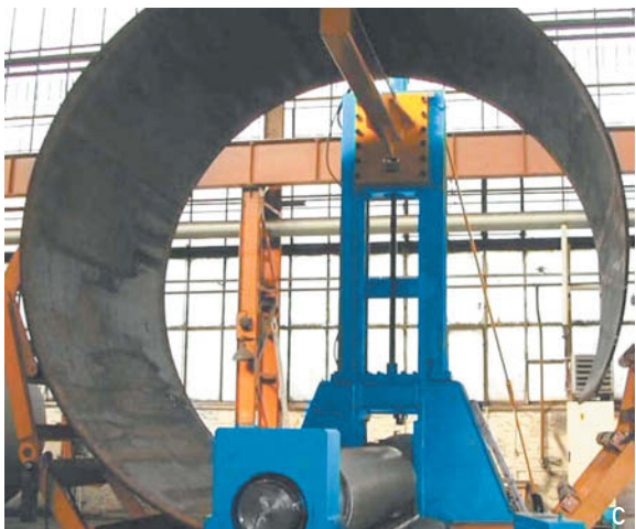
Figs. 3A-C: Three stages in the plate-bending process.
