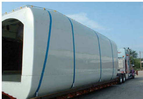
Fig. 1: Nacelle housing.
