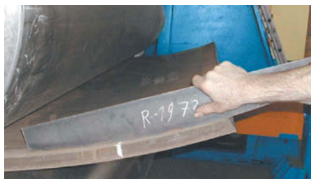
Fig. 4: The trailing edge of the plate is prebent in the same manner as the leading edge.
