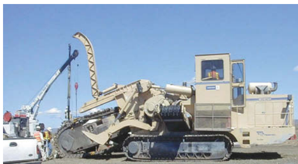
Fig. 6: Maintaining the chain trenching machine.
